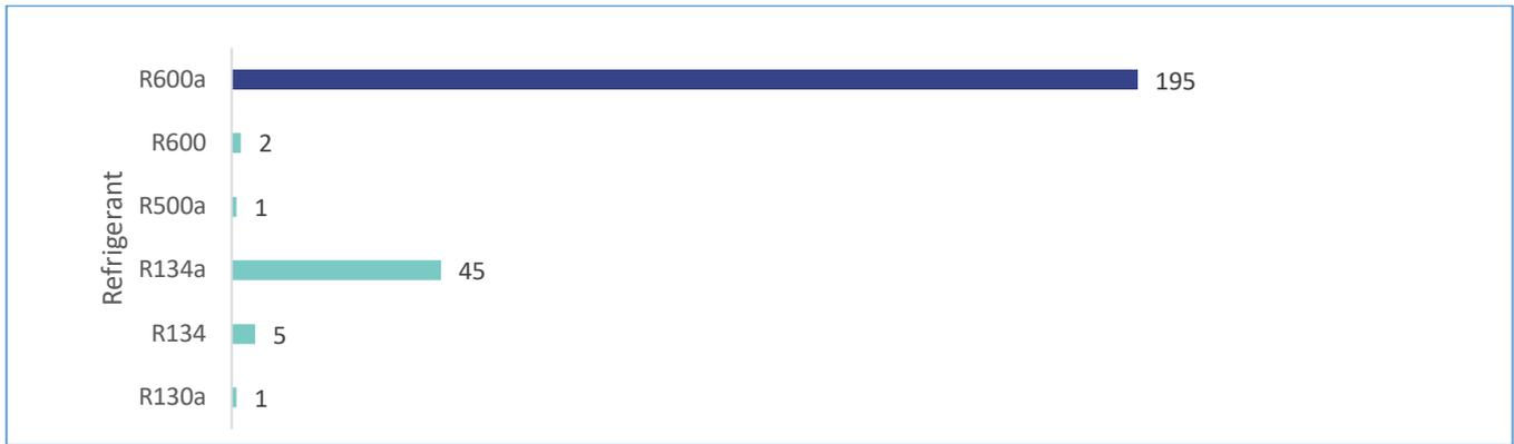
Figure 10: List of Refrigerants used in Zambia as informed by the survey (Source; Residential Refrigerators Survey 2021).
